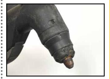
Regularly inspect your consumables for wear. Replace when excessive wear is apparent.
