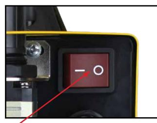
Plug the machine input power lead into the 15 Amps wall socket, ensuring that the Mains Power Switch is OFF.
