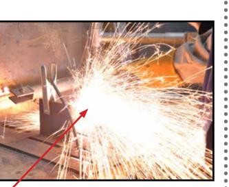
If the sparks a blown out toward the torch or at a great angle below the work piece, reduce the cutting speed.
