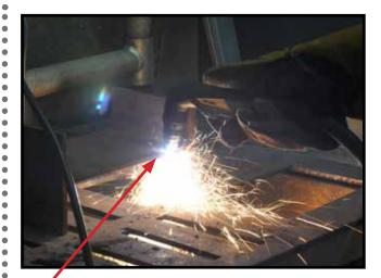
At the end of the cut pause to allow the plasma to sever the last part.
