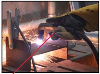
Depress switch and the pilot arc fires from 10 the nozzle and care must be taken when depressing trigger switch. This arc is designed to burn through contamination, paint or rust to allow the main cutting arc to connect with bare metal. Continued depressing of the switch away from cutting surface will reduce the effectiveness of the consumables and greatly reduce their life span.
