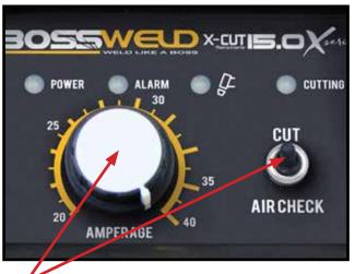
Select your required current turning the 8 Current Adjustment Knob. If the plasma is struggling to penetrate, increase amperage by turning the Current Adjustment Knob Set the CUT / AIRCHECK switch to CUT,
