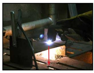
Adjust the cutting speed so that the sparks go through the work piece and out the bottom of the cut.
