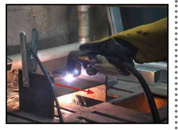
After the cutting arc starts, slowly start moving the torch across the work piece. **Note:** Always start the Arc on a material edge or drill a small hole in the work piece to start Arc.
