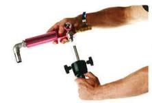
**5.** Screw the CIMFLO® Regulator body to the adjustable suction pipe (5).
