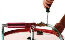
8. Attach and tighten hoses and clamps. Other hoses of comparable size can be used. (Not supplied).
