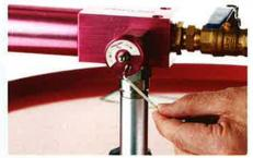
**12.** Using a hex or Allan Key (not supplied) tighten the grub screw to lock in the set mix.
