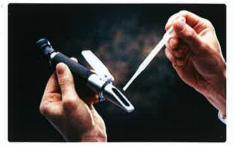
Check the concentration, use a refractometer or alternative method of determination.
