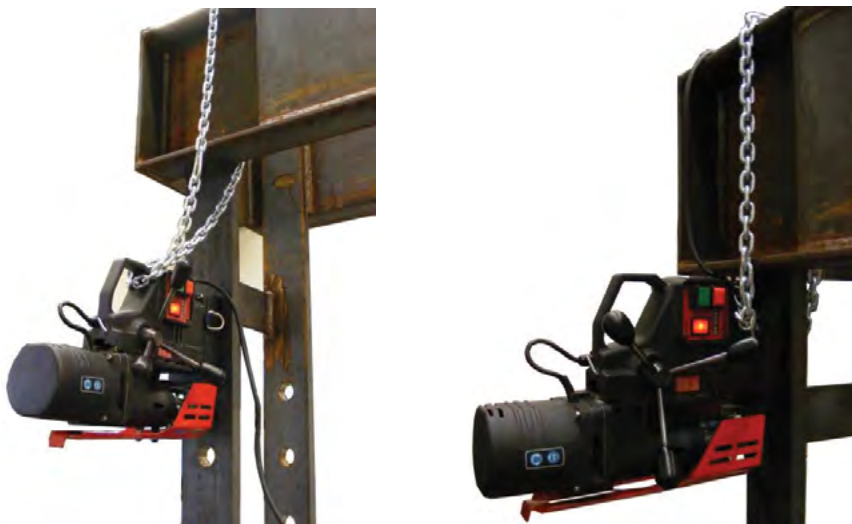
Fig. 1 An example of a safety chain/strap use.
