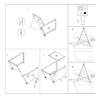
If the machine needs to be moved in its own packing, use a forklift truck or sling it with straps as illustrated in drawing 6 above.
