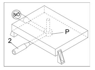
To move the vise in either direction, the vise jaw must be unlocked at two points.
