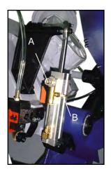
The hydraulic cylinder is ideal for the cutting of thin or STAINLESS STEEL section bars, that determines a constant lowering and consequently a good efficiency of the blade throughout the work phase. By adjusting the flow control valve (A), this device can be accommodated to the different situations and applications. Defectiveness in the control of the lowering may be caused by the drop in braking power of the device due to the long-term blowby of the braking fluid.
