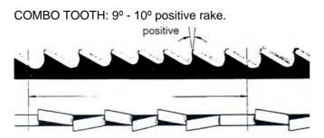
This type of blade is the most suitable for the cutting of section bars and large and thick pipes as well as for the cutting of solid bars at maximum machine capacity. Available pitches: 3-4/4-6.
