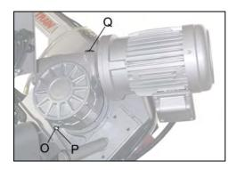
The gear box requires periodic changing of oil. The oil must be changed by the first 6 months of a new machine and every year thereafter.
