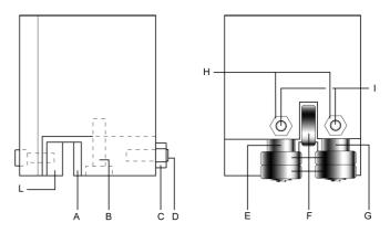
In case the blade needs to be replaced, make sure to always install 0.9mm thick blades for which the blade guide pads have been adjusted. In the case of toothed blades with different thicknesses adjustment should be carried out as follows:
