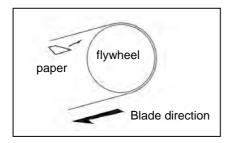
Use a strip of scrap paper and slide it between the blade and the flywheel while it is running. -if the paper is cut then the blade is riding too close to the flange. Re-adjust.
