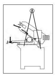
To move the machine, the machine needs to be moved in its own packing, use a forklift truck or sling it with straps as illustrated in the drawing above.
