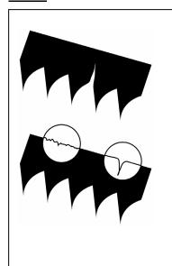
Blade guide pads not regulated or dirty because of lack of maintenance
