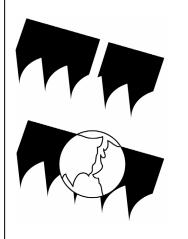
Faulty welding of blade
