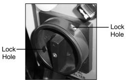
The main connect switch is designed with a lock hole. A lock can be used in the lock hole to prevent operation of the machine for safety or security.
