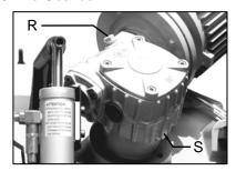
The gearbox requires periodic changing of oil. The oil must be changed by the first 6 months of a new machine and every year thereafter.
